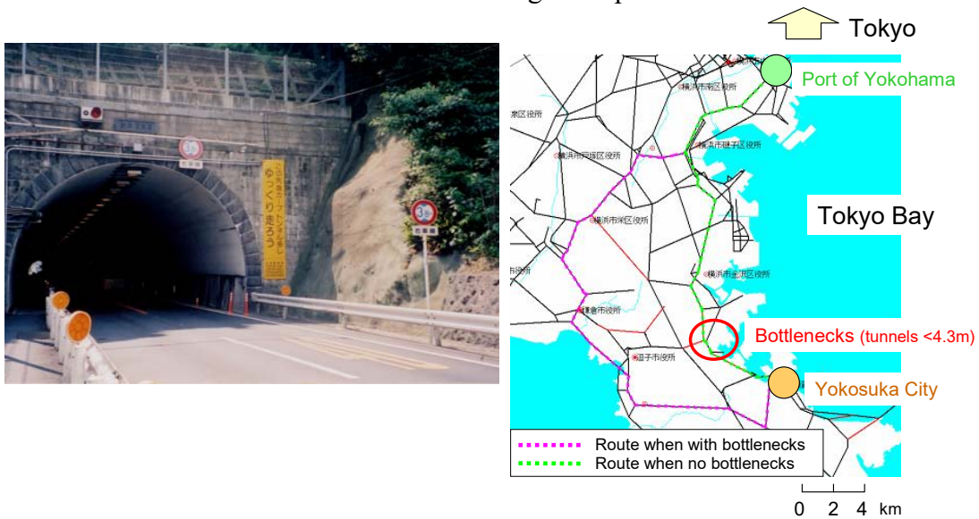
Fig. 8 Sample of bottleneck for semi-trailers for high-cube container and detour route (in case of no use expressway)
